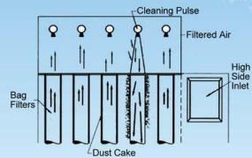
Inside Look of Ultra-Flow Cleaning Dirty Air Debris and Fumes Drawn Up Through the Bag Filters for Maximum Indoor Air Quality
