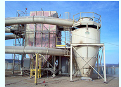
Old technology collector retrofitted to new technology and corrected severe moisture compacting dust and freezing in winter.
