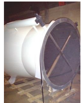
BOOSTER cleans spark arrestor cell
